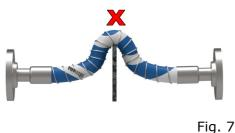
**INSTALLATION:** The hoses must be supported to allow normal movement when under pressure (dimensional variations).
