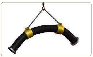
For transportation, installations or support in place, never use a single rope to lift hose.
