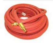
A good-quality, economical general purpose hose for industrial air service, compressor lines, pneumatic tools, low-pressure spray,and many other applications where the need for oil resistance is moderate. Non-conductive, minimum electrical resistance greater than one (1) megohm per inch of hose length at 1000 volts DC. Available in 200 and 300 psi working pressures, with a temperature rating of -20°F to 190°F (-29°C to 88°C).
