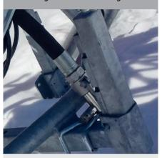
The extremely robust hose barb adapters are used above all for stationary long-term installations of pipe and hose lines.
