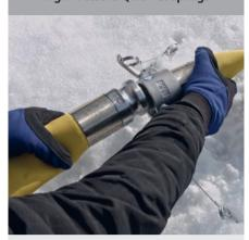
These special couplings are particularly suited for snow and pump machines, tunnelling, conveyor technology or other high-pressure applications with liquids.
