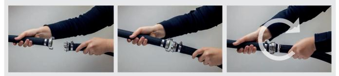
GEKA plus claw couplings are connected the same way as standard claw couplings. Push the two couplings together at 180° degrees opposite to each other until the seal faces touch. Afterwards, rotate one coupling half as far as it will go into the opposite direction of the other - the couplings lock into place.
