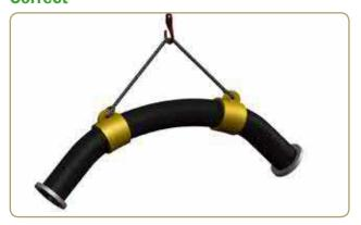
For transportation, installations or support in place, never use a single rope to lift hose.
