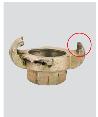
Counterfeit from the Far East (no manufacturer's branding, inferior material)
