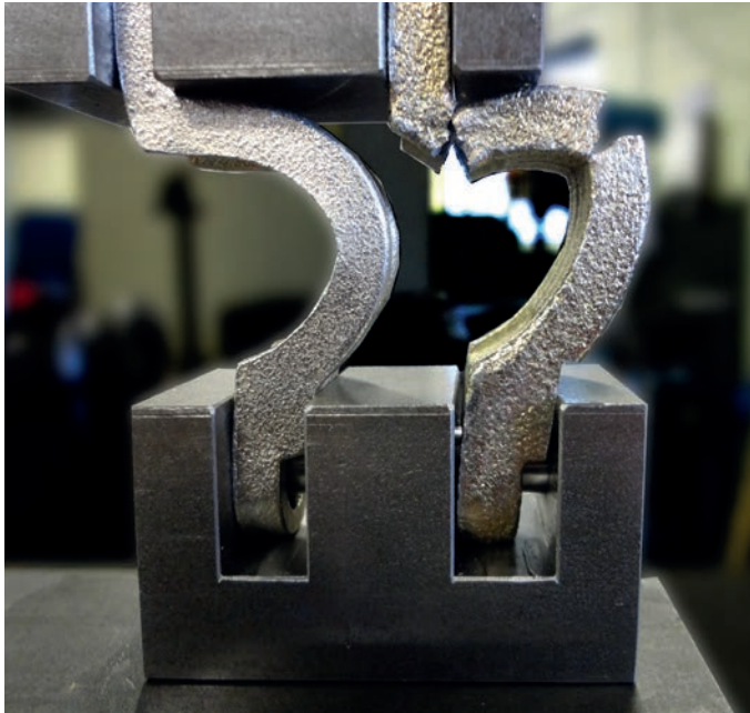
Fracture test - left: LUDECKE hose clamp (no crack/ fracture), right: hose clamp from the Far East (complete fracture)
