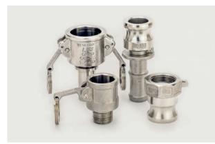
Kamlok quick couplings are extremely robust couplings to connect large volume hoses to each other or plants. In this asymmetrical coupling system, a male and female part is locked by two handles.
