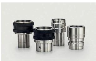
The **LUDECKE** SoftFlow material conveying quick connect couplings are a high-quality quick coupling system for pressure and vacuum conveying of bulk material or liquids (e.g. for vacuum-conveying granulate). Due to their quick coupling principle with ball shut-off and light weight, the couplings are especially easy to handle. The coupling body is made of stainless steel for less abrasion.
